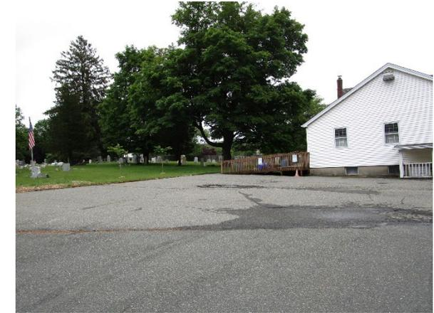
Pervious pavement can be installed south of the building near two disconnected downspouts to capture and infiltrate stormwater runoff from the parking lot and building. Parking spaces in the north parking lot can also be retrofitted with pervious pavement. A preliminary soil assessment suggests that the soils have suitable drainage characteristics for green infrastructure.
